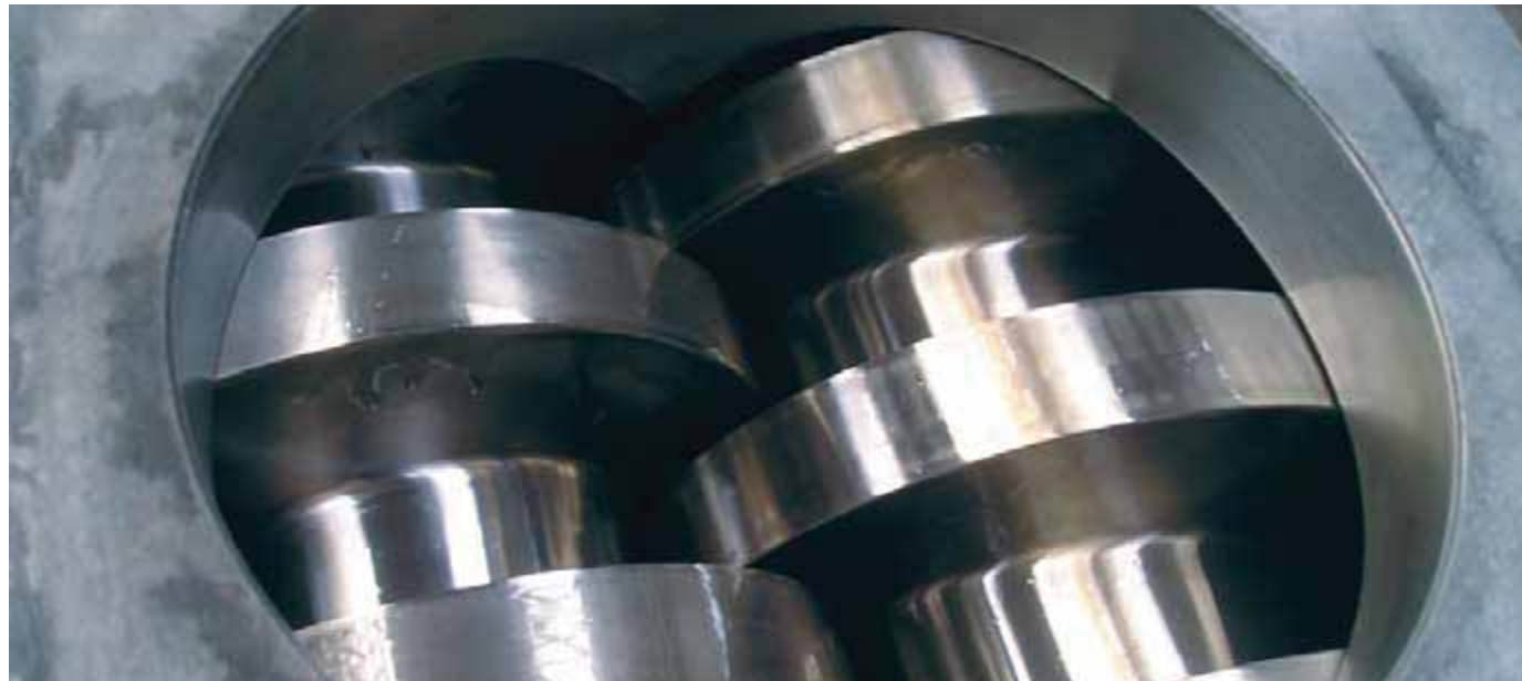
Conical interlocking screws (a complicated technical solution in the machine)
